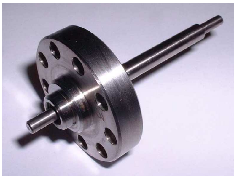
Figure 3.5: A photograph of an ISUK which consists of a 1 mm diameter optical fibre mounted within a custom-made titanium vacuum feedthrough.
