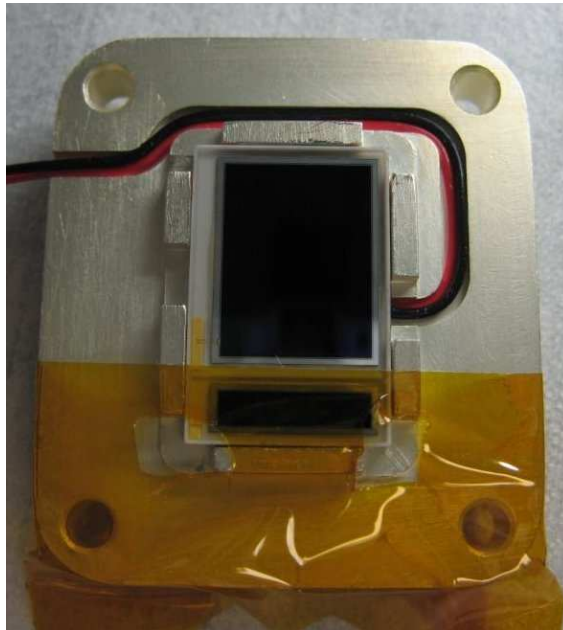
Figure 2.1: A production photograph of one of the PIN diode packages mounted on one of the copper shield walls, temporarily held in place with Kapton tape. To prevent oxidation, the copper shield pieces are coated with a silver layer several microns thick. Note the sensitive silicon part of the diode (black) is laterally offset from the centre of the substrate. Photograph courtesy of IEEEC.
